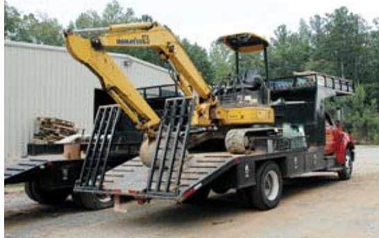
Pine Enterprises designed its own trucks, eliminating the need for a trailer, to transport its Komatsu compact excavators.
