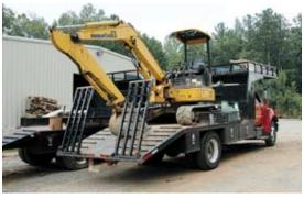
Pine Enterprises designed its own trucks, eliminating the need for a trailer, to transport its Komatsu compact excavators.
